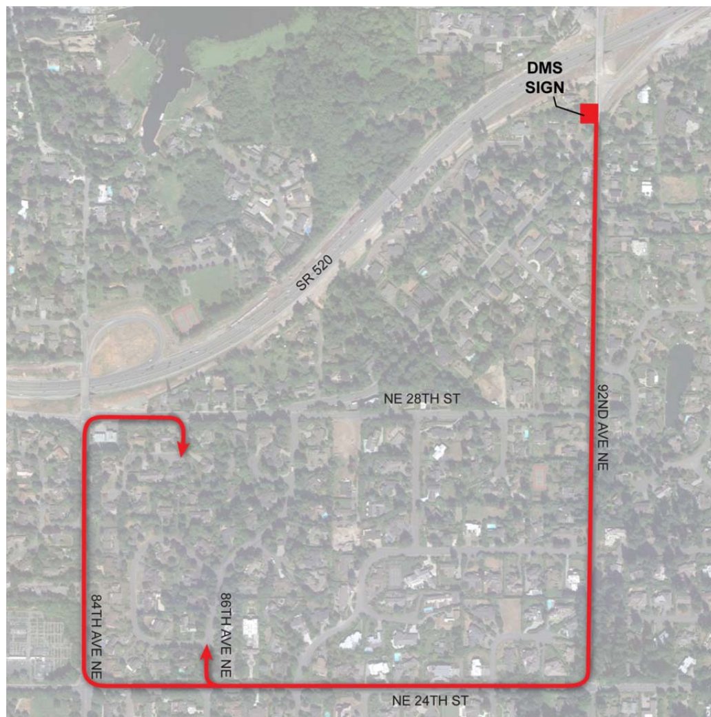
Figure 5: Provide advanced warning signs at 92nd Avenue NE
